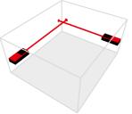
Min./max. measurement You can find out both minimum and maximum distances by measuring the shortest distance between 2 points or the longest distance, such as a diagonal.
