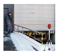
Pulse function: With a hand-held receiver, it is also possible to use the CROSSLINE outdoors, at distances of up to 80 m. This means it has one of the longest ranges among crossline lasers of its kind.
