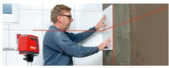
Its clearly visible horizontal and vertical laser lines form a cross with an angle of exactly 90°.
